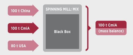
Under the mass balance system, quantity control is undertaken at the spinning mill level. An online tracking system developed for Cotton made in Africa controls the amount of cotton bought and balances this with the amount of thread sold. If a spinning company experiences a shortfall in the material balance, it must then promptly buy the missing amount of Cotton made in Africa cotton.
